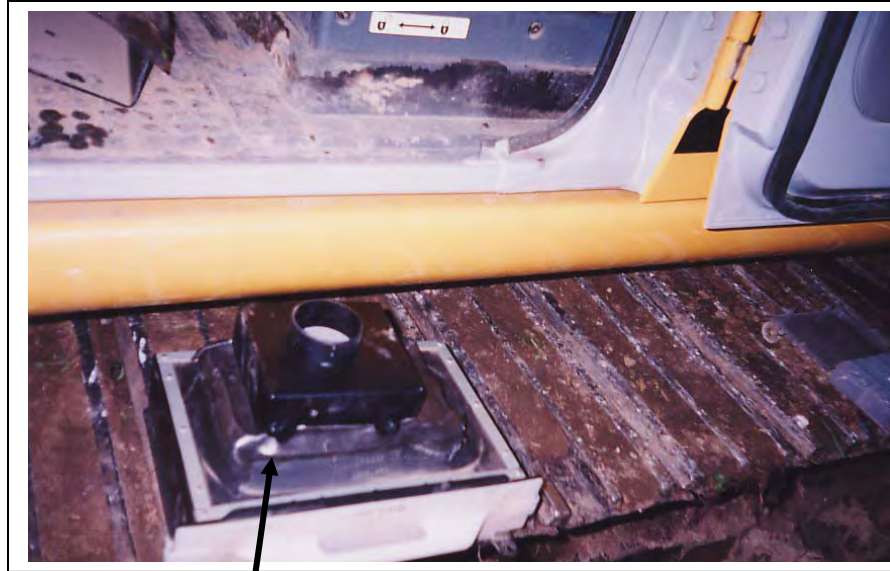
Outside air filter assembly with outside air intake box mounted and ready for reinstallation.
