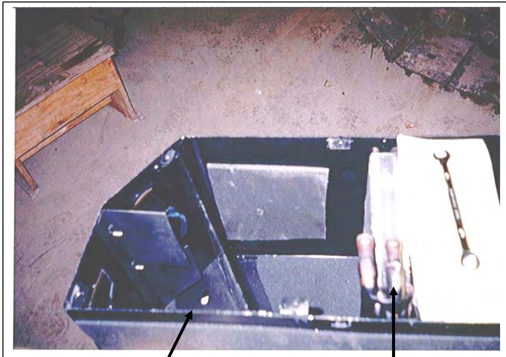
Right hand side mounting hole. Access by removing box lid.
