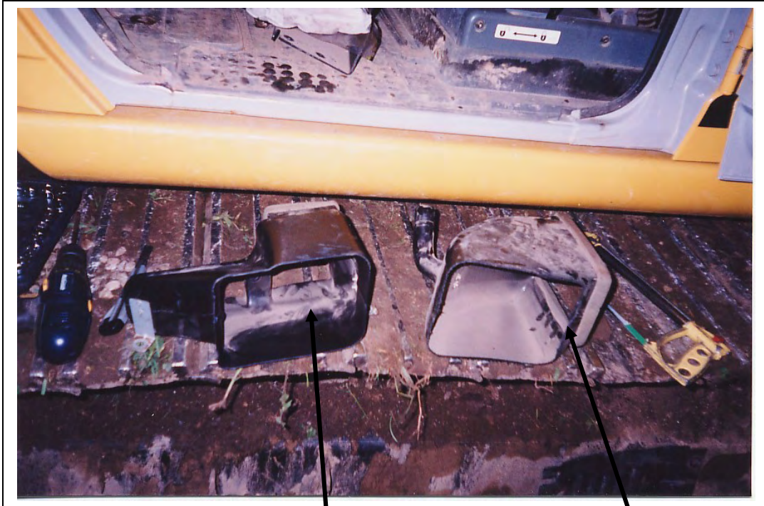
Retain and reinstall after the heat/cool box has been mounted. Seal to the box with tar tape and self adhesive foam tape. Cut with a knife or hack saw. The retained section is approximately 6" long
