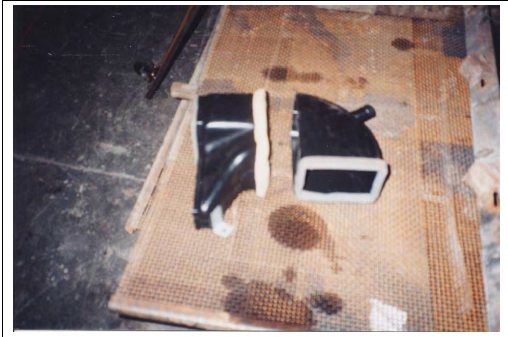
1" x 1" foam tape installed around front air duct piece where it will seal to the new AC box.
